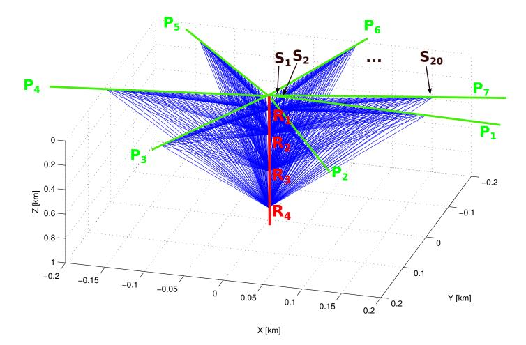
20 sources  $S_i$  on 7 surface profiles  $P_i$  and 4 receivers  $R_i$  in the borehole
