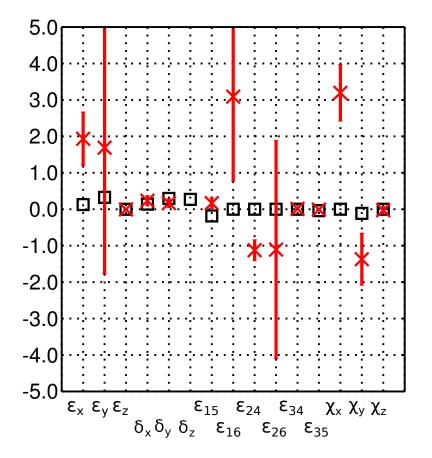
Model A4, 5 ms noise; black squares - exact, red crosses - inverted values, red bars - estimated errors of WA parameters
