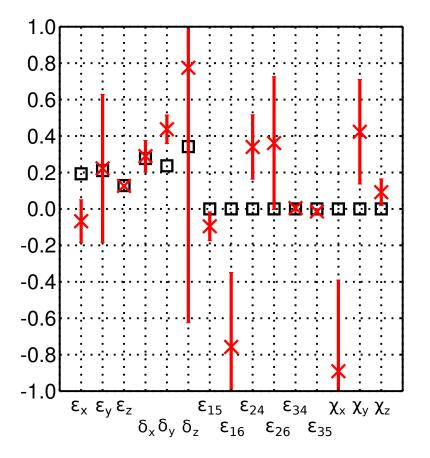
Model A1, 5 ms noise; black squares - exact, red crosses - inverted values, red bars - estimated errors of WA parameters
