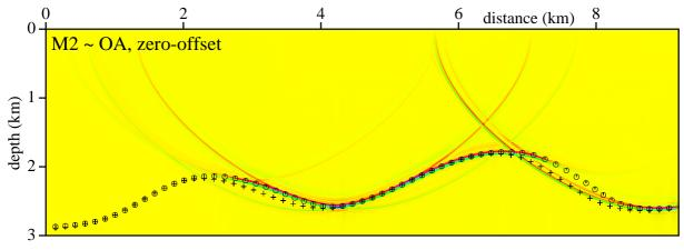
• We continue with the second iteration towards velocity model used for migration and determine mean values (M2) of rotated elastic moduli (M1) and elastic moduli for migration (OA) without rotation.
