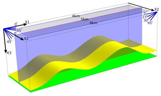
• For calculation of the recorded wave field we use velocity models with orthorhombic, VTI or triclinic anisotropy, all with differently rotated tensors of elastic moduli in the upper layer. The angles of the rotation are 15, 30 and 45 degrees around axes  $x_1$ ,  $x_2$  or  $x_3$ .
