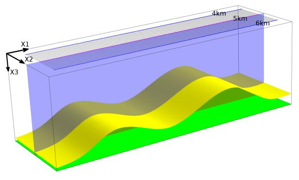
• The 3-D measurement configuration consists of 81 parallel profile lines, the interval between the parallel profile lines is 0.025 km.
