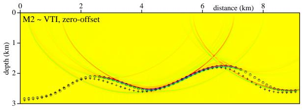
• We continue with the second iteration towards velocity model used for migration and determine mean values (M2) of rotated elastic moduli (M1) and elastic moduli for migration (VTI) without rotation.
