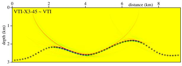
• Stacked migrated sections calculated in the incorrect velocity models with VTI anisotropy without the rotation of the tensor of elastic moduli. The correct anisotropy is VTI with 45 degree rotation of the tensor of elastic moduli around the  $x_3$  axis (VTI-X3-45) that is due to symmetry the same as without rotation (VTI).
