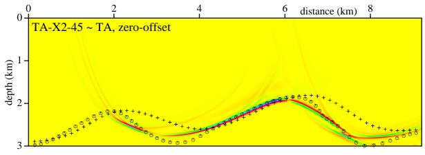
• Zero-offset stacked migrated sections calculated in the incorrect velocity models with orthorhombic anisotropy (TA) without the rotation of the tensor of elastic moduli. The correct anisotropy is orthorhombic with 45 degree rotation of the tensor of elastic moduli around the  $x_2$ axis (TA-X2-45)
