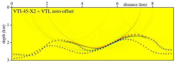
• Zero-offset stacked migrated sections calculated in the incorrect velocity models with orthorhombic anisotropy (VTI) without the rotation of the tensor of elastic moduli. The correct anisotropy is orthorhombic with 45 degree rotation of the tensor of elastic moduli around the  $x_2$ axis (VTI-X2-45).
