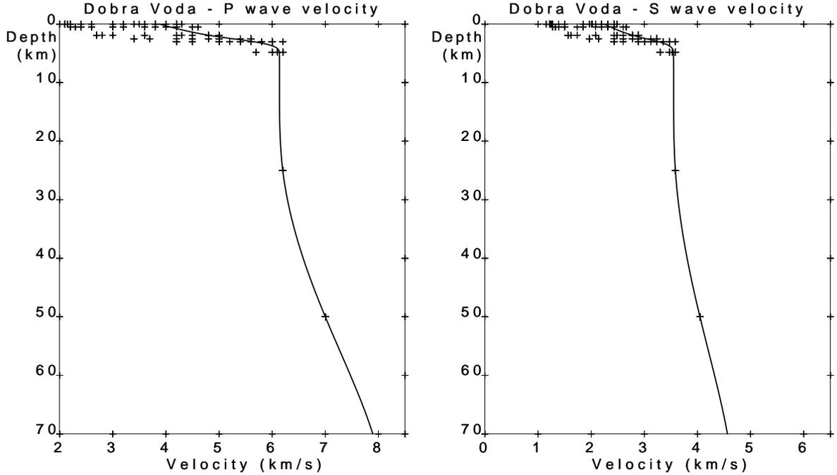
**Figure 1:** 1-D P-wave (left plot) and S-wave (right plot) velocity models of Dobrá Voda locality. The vertical axis is the depth, horizontal axis is the P-wave or S-wave velocity. The crosses show the values of the velocity in the data points. The solid line shows the velocity in the constructed smooth 1-D velocity models.
